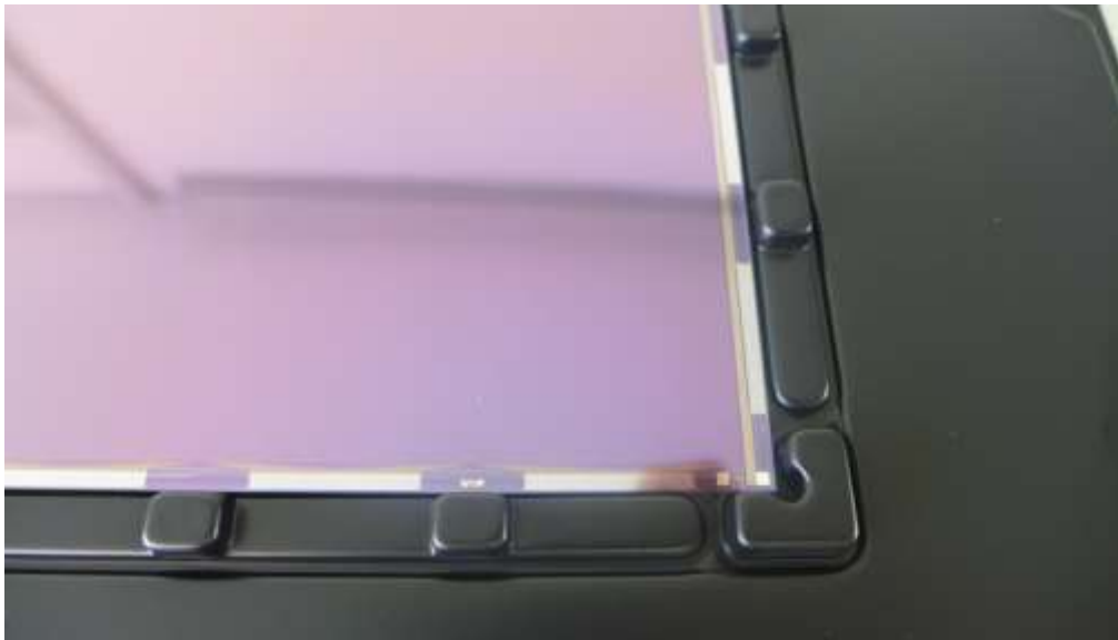
Electronic glass panel (LCD, sensor, etc.) Interconnects pitch = 0.2 mm
